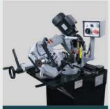
CAST IRON SWIVEL BOW HEAD AND QUICK ANGLE ADJUSTMENTS UP TO 60°
